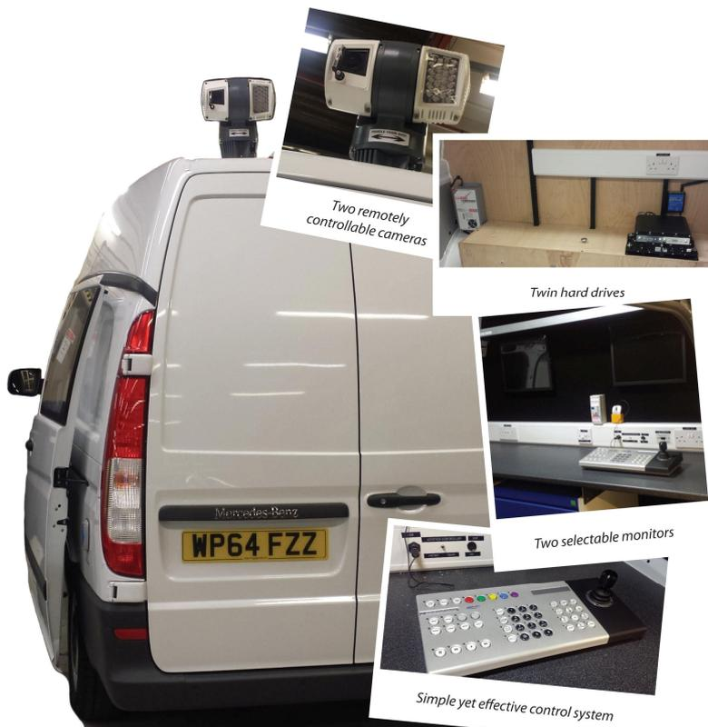
The Van is a High Top Mercedes Vito van with a viewing room separate from the front drivers area and a separate area for batteries and Hard drives
